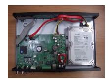
3. Hold the HDD in place, and use a screwdriver to fix it.
