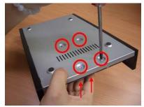
4. Replace the device's cover and the securing screws.
